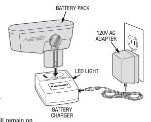
3. When fully charged, reattach battery pack onto Cordless Circular Saw, making certain latches fasten securely. Cordless Circular Saw will not operate properly if the battery pack is not seated properly.
